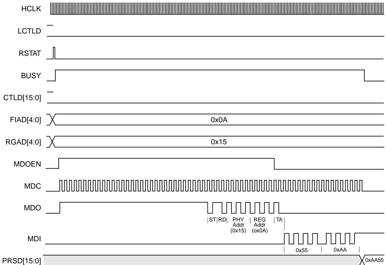
The timing shows the sequence of events to read from a PHY status register. The values used for data and address are illustrative only, and
