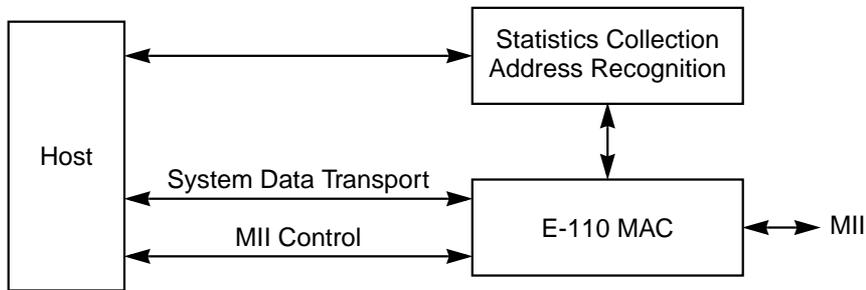
For simplicity of application, all per packet interactions (for example, start of frame and end of frame) between the E-110 MAC and the system take place through the system data transport. Using the system data transport eliminates the need for involvement of a processor at 100 Mbit/s because the E-110 MAC takes over the per packet data transfer responsibility.
