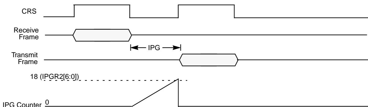
When instructed, the transmit function adds a preamble and SFD to the supplied packet data and, if requested, appends a generated FCS. The E-110 MAC transmit function adds bytes of zero before the appended FCS to pad packets with fewer than 60 data bytes. The transmit function detects and enforces collisions with jams and manages transmission retries.
